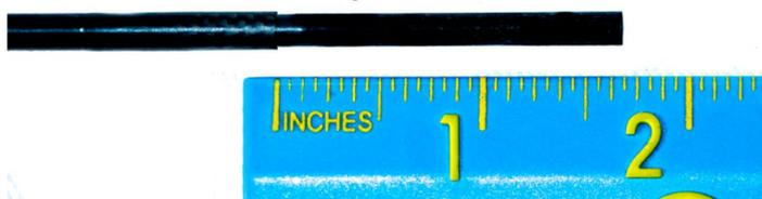
Figure 5: This gives a good indication of how much overlap there is between the two sections when they are fitted together conventionally. If this distance is too short - there can be problems and weakness.
