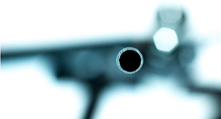
Figure 2: Not the worst example - but there is a marked difference in wall thickness in this prototype test-blank. The more you pay for a rod - the better this aspect needs to be. This one was sent back for improvements to manufacturing process on a premium rod.
